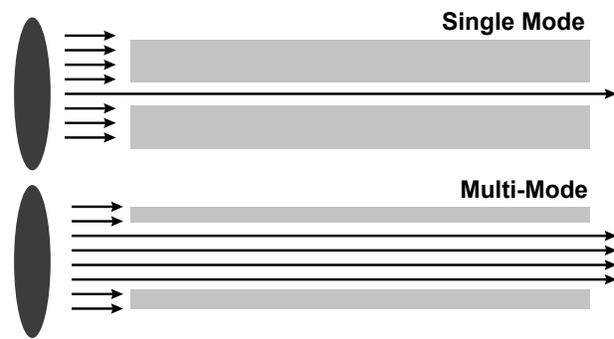
Fig. 5 - LED into Single Mode vs Multi-Mode Fiber
