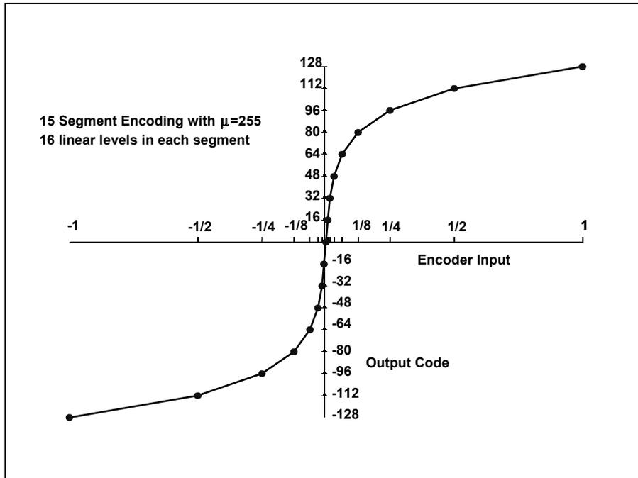
Figure 9 -  $\mu$ -law Quantizing/encoding
