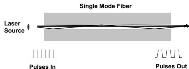
Fig. 7 - Dispersion for a Single Mode Fiber
