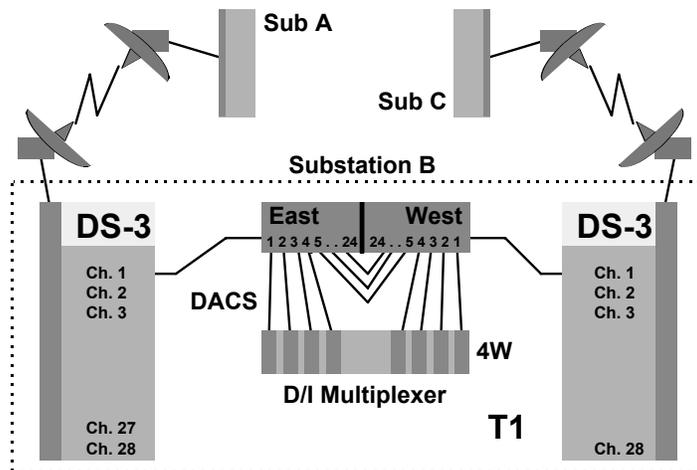
Figure 12b - Typical Microwave with D/I Multiplexer Application
