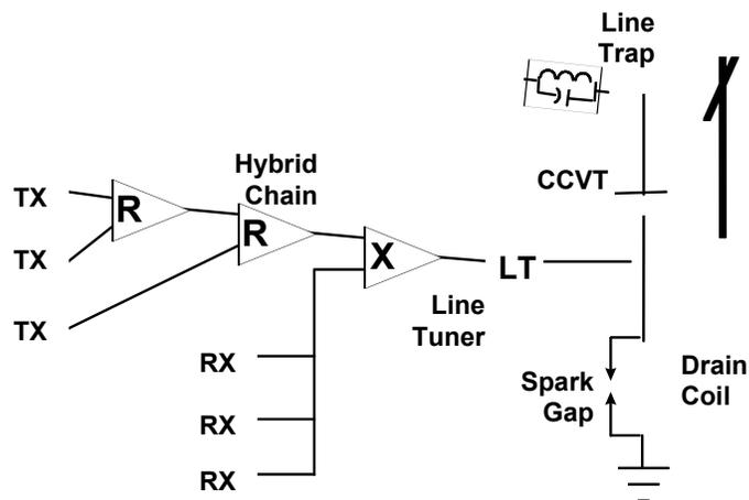
Figure 2 - Typical Power Line Carrier Terminal
