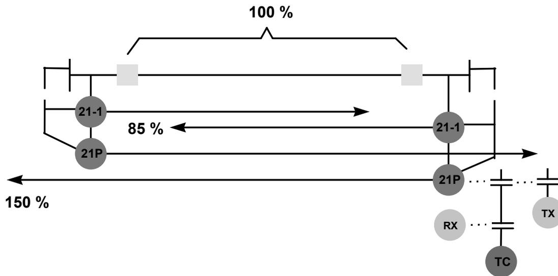
Figure 1 - Basic Distance Pilot Relay System
