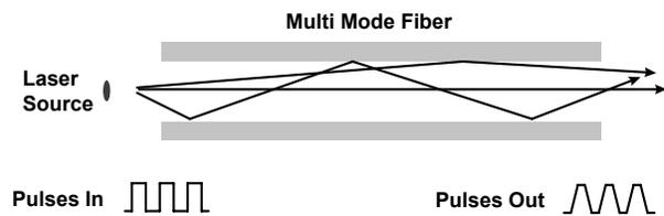
Fig. 6 - Dispersion for a Multi-Mode Fiber
