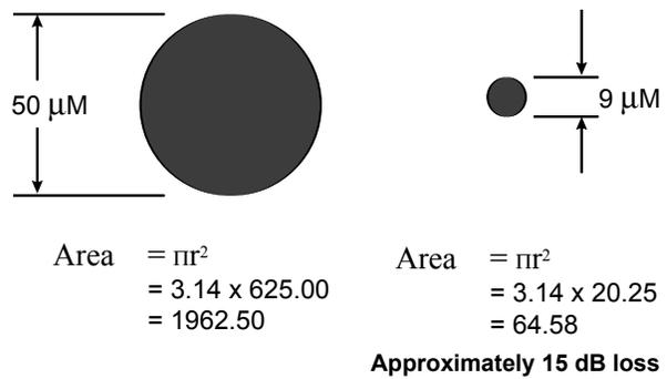
Fig. 4 - LED vs Laser
