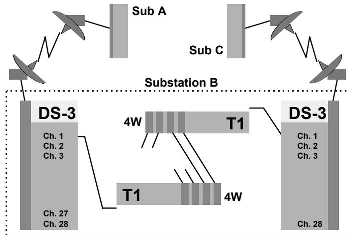
Figure 12a - Typical Microwave with Pt to Pt Channel Bank Application
