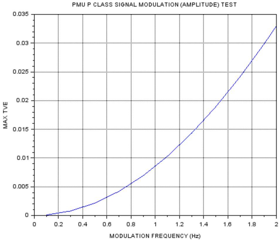
**Fig.2:** TVE vs Modulation frequency plot for the P class reference design (0.1 – 2 Hz)
