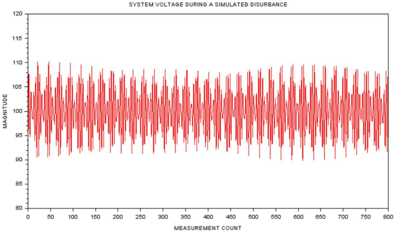
**Fig.8:** Phasor magnitude of the system voltage during a simulated disturbance
