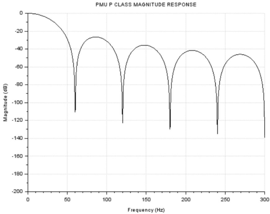
**Fig.6:** Magnitude response of the P class reference filter
