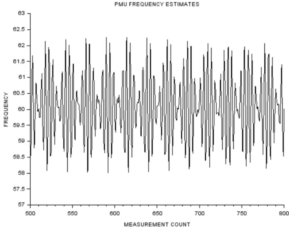
**Fig.10:** Frequency estimated by the P class reference filter during a simulated system disturbance
