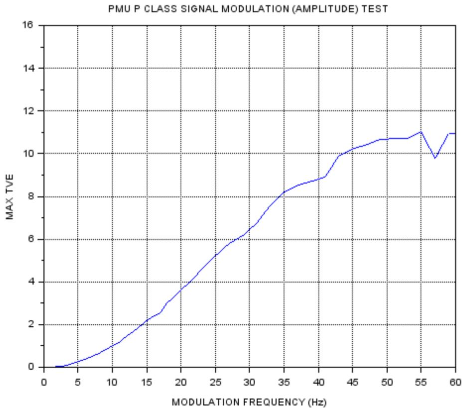
**Fig.3:** TVE vs Modulation frequency plot for the P class reference design (0 – 60 Hz)
