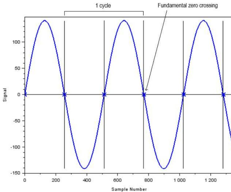
**Fig.1:**  $U_{rms(1/2)}$  measurement technique
