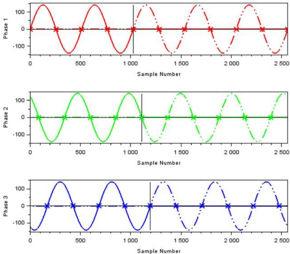
**Fig.4:** Representation of test 6.4.2 of the IEC 62582-2 - Check dips / interruptions in polyphase system
