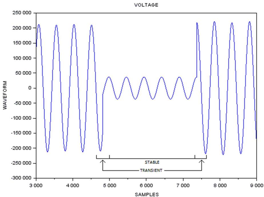
**Fig.3:** Voltage dip with a non-zero incidence angle
