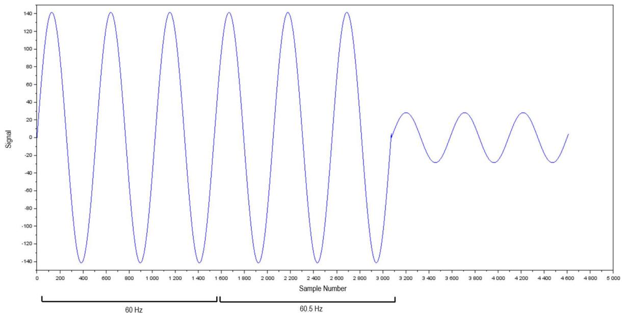
**Fig.2:** Voltage dip after a fluctuation in the system frequency
