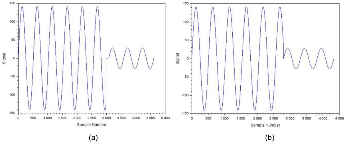
**Fig.5:** Voltage dip - (a) Temporary loss of phase (b) Permanent phase shift
